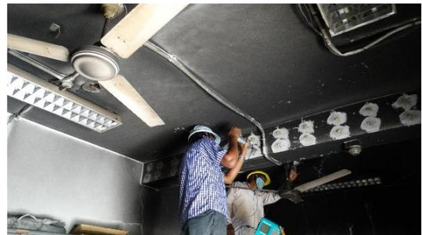
Fig.4a : Typical view of Rebound Hammer Test in ground floor
