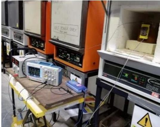
**Figure 3** : Measurement system using GMR sensor Temperature vs Time
