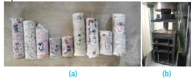
Fig.8 : (a) Extracted Concrete Samples
