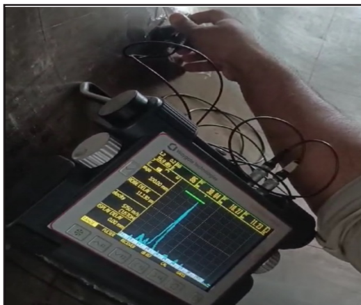
Figure 10: Flaw picked with conventional focused T-R probe during inspection from cladding surface
