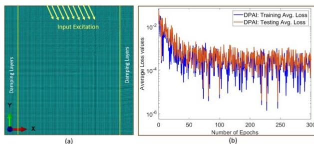
**Figure 7:** (a) FE modeling: all the active aperture elements are triggered in parallel using pre-defined delay laws to form the ultrasound beamforming to steer in the medium. (b) DPAI: Training/Testing: the average loss values over a number of epochs for phased array beam steering datasets.
