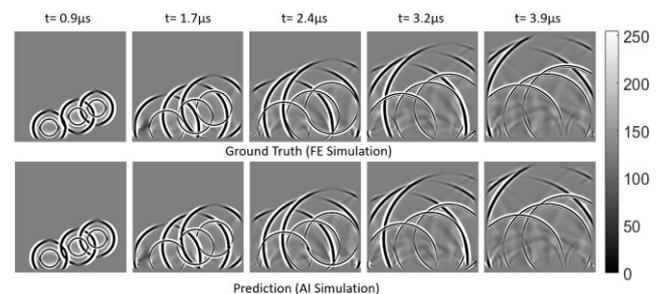
(a) Comparison between AI/FE simulation for the single excitation source.
