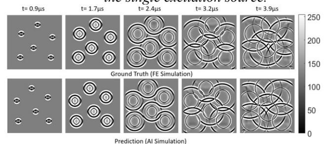
(b) Comparison between AI/FE simulation for four excitation sources
