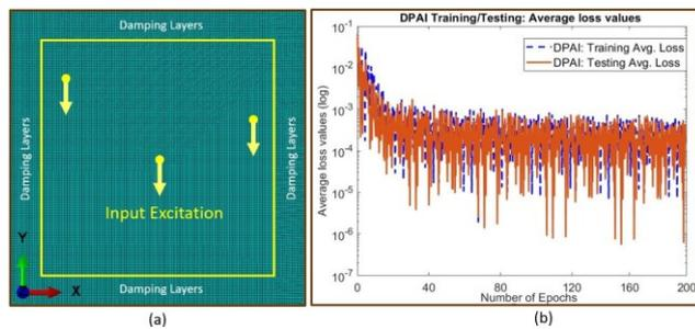
**Figure 2:** (a) An example of the FE model, where the incident wave is triggered by modelling the three excitation point sources. The absorbing boundary condition is applied to all wall sides with different damping coefficients to prevent undesirable effects.
