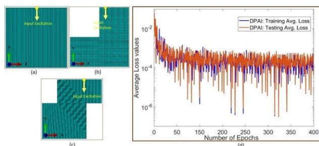
**Figure 5:** (a) Finite element models: To create the training dataset, FE models with single point sources are excited in the Y direction at the top surface of the domains. (b) DPAI: Training/Testing: The model was trained using the reflection from the boundary datasets, the model average training, and the testing loss throughout the number of epochs.
