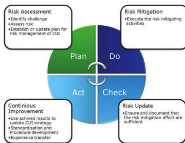
Fig.1 Corrosion under insulation plan-do-check-act approach to achieve asset integrity [7]
