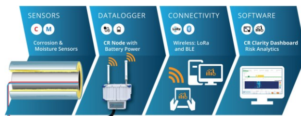
Fig 4 CorrosionRADAR CUI monitoring system and different arrangements of the sensor appropriate for different piping or vessel types as well as the node that is capable of sending the data to the cloud.
