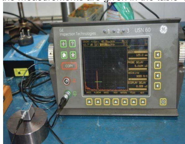
Fig4: Ultrasonic velocity measurement on specimen with USN60 equipment
