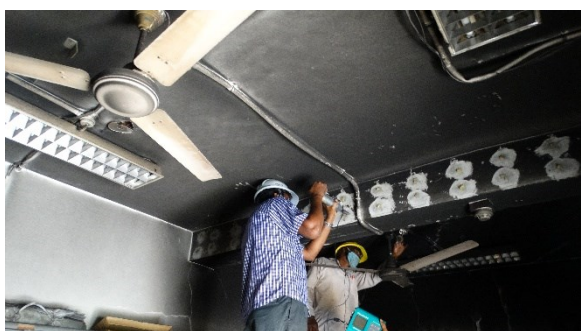
Fig.4a Typical view of Rebound Hammer Test in ground floor
